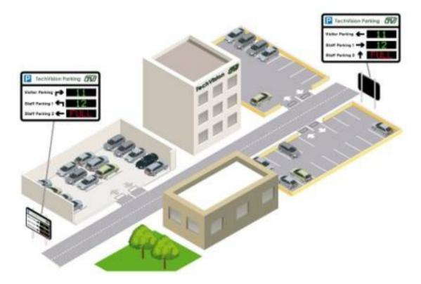
Nortech's NorParc© PC-based car park count management system supports a range of Nortech's vehicle detection and counting products to monitor the availability of free parking bays over multiple car parks and provide guidance to customers as they arrive to search for available spaces.
