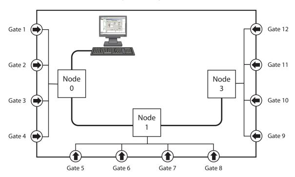
Keep a record of the node identity of each NCT200 module together with the location of the monitored access point to which each of the counters relate. If possible, mark up a plan of the venue with the positions of the NCT200 modules and mark the node and counter number (from 0 to 3) against each of the associated access points (for example '4-0' shows that the counter is counter 0 of node 4).
