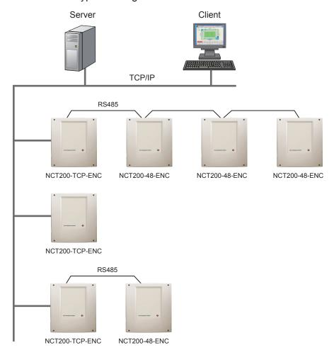
Each thin server needs to be assigned a valid IP address and a port number. The IP address may either be automatically assigned by a DHCP server on the network, or, where there is no DHCP server, manually using the Lantronix utility program to access the thin server over the network.
