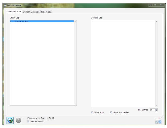
This screen will show communications activity when the Server is running. The left-hand panel displays communications activity with the Client software and the right-hand panel displays communications activity with the counter modules.
