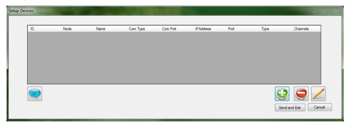
Initially, no devices are shown. Add each device one at a time by clicking the '+' button and entering the data in the 'Setup Device' box.
