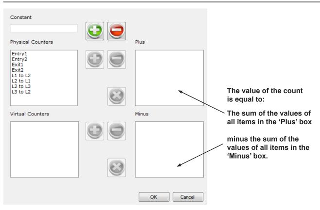
Counters can be added to either box according to the required formula for the virtual counter. For example, to create the formula 'Entry1' minus 'Exit1':
