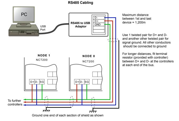
The connection to the PC is via a USB/RS485 converter (supplied). This must not be plugged into a USB port on the PC until the Server software has been loaded, as the correct driver for the converter is loaded with the Server software.
